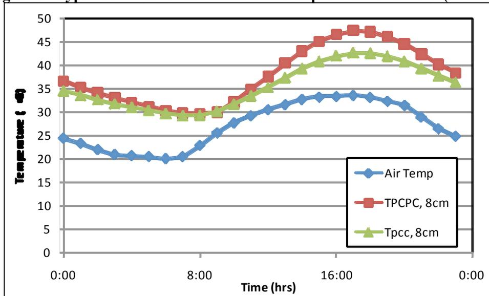
The temperature behavior of the PCPC system with depth is shown in Figure 3 for the same time period shown in Figure 2. The changes in the PCPC temperature followed closely behind the air temperature variations, and temperatures fluctuated less with depth. The 60 cm depth fluctuated less than  $1^\circ\text{C}$  over the analyzed time period.
