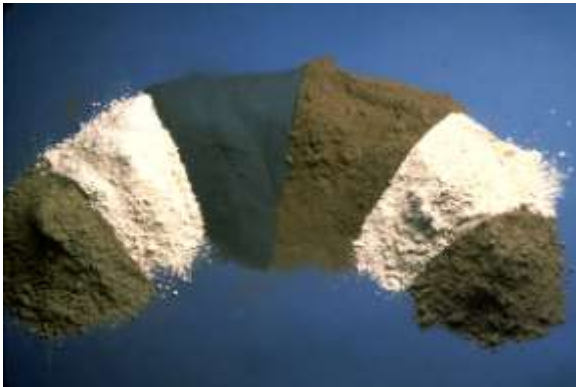
Supplementary cementitious materials. From left to right, fly ash (Class C), metakaolin (calcined clay), silica fume, fly ash (Class F), slag, and calcined shale.
