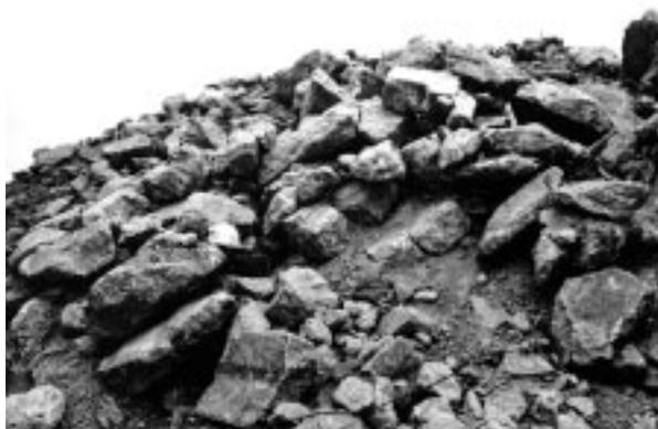
Figure 11. PCC stockpile for recycling. (S-42546)
