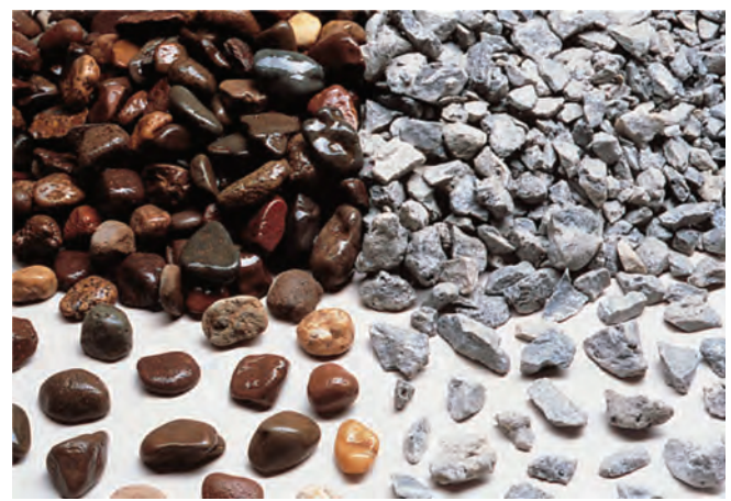
Figure 4.7 Rounded (left) and crushed natural aggregates (photo courtesy of Portland Cement Association)
