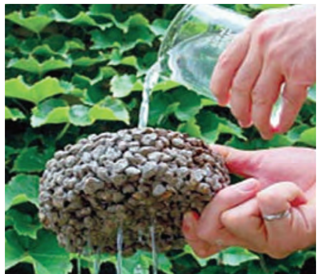
Figure 9.3 Water passing through pervious concrete (NRMCA 2009)
