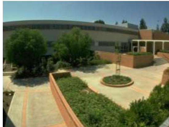
Increasing the amount of high-albedo materials and implementing non-roof heat-island reduction techniques such as using light-colored concrete for walkways and landscaping may help contribute toward gaining an Innovation Credit.
