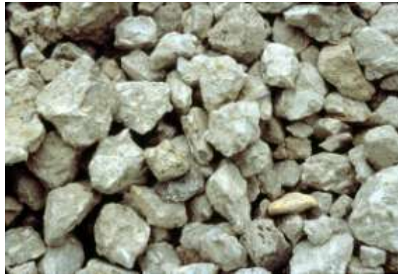
Concrete taken from demolition sites may be recycled by crushing and reuse as backfill or as a base for road construction.
