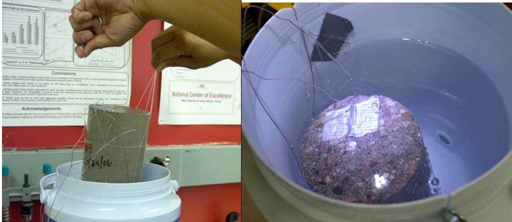
Figure 39 a) Immersing heated specimen into insulated flask. b) View of fully immersed specimen as it reach equilibrium with water temperature.
