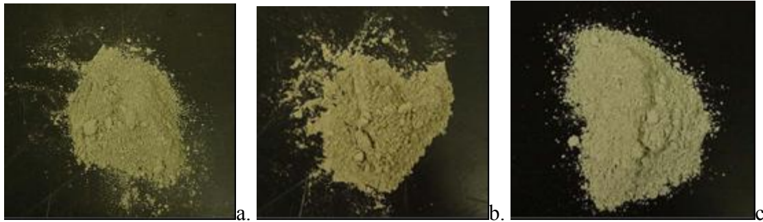
Figure 12 Three cementitious materials used in concrete. a) Portland cement (cement), b) flyash (FA) c) ground granulated blast furnaces slag (slag).
