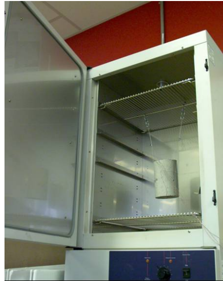
Figure 38 Convective oven used for heating suspended material specimens.
