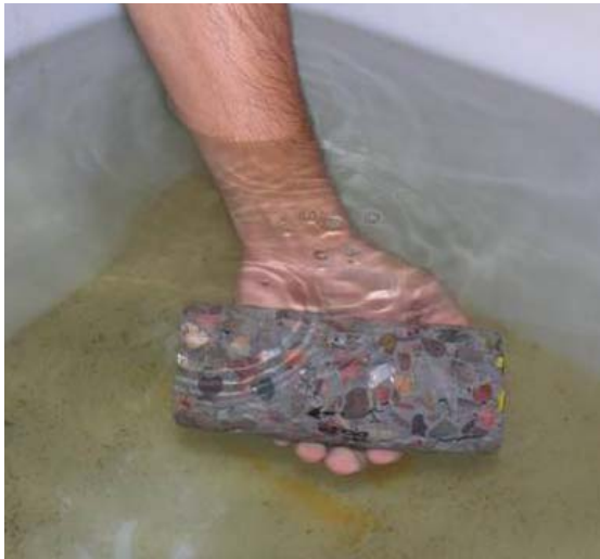
Figure 31 It is important to remove trapped air from within sample until completely saturated.
