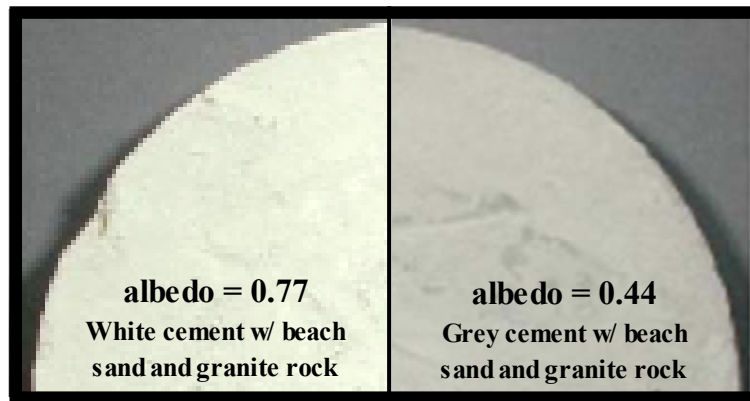
Figure 7 Albedos of white and grey cement with identical aggregate proportions. Source: Levinson and Akbari, 2001
