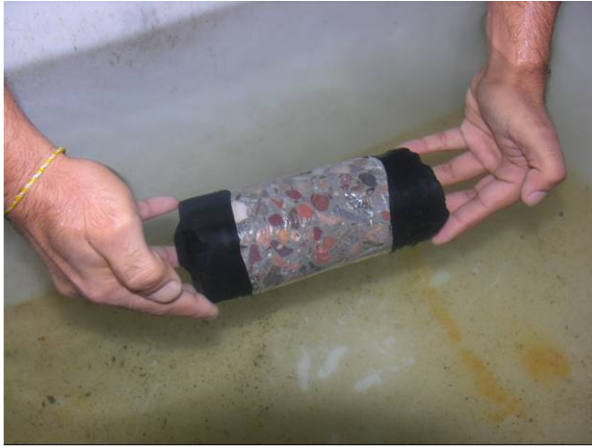
Figure 33 A sample is sealed underwater using polystyrene and elastic rubber caps.
