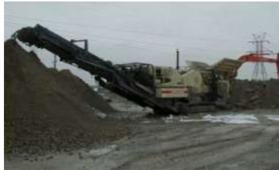
Crushing concrete and then using the material for aggregate is an opportunity to qualify for recycled content credit.
